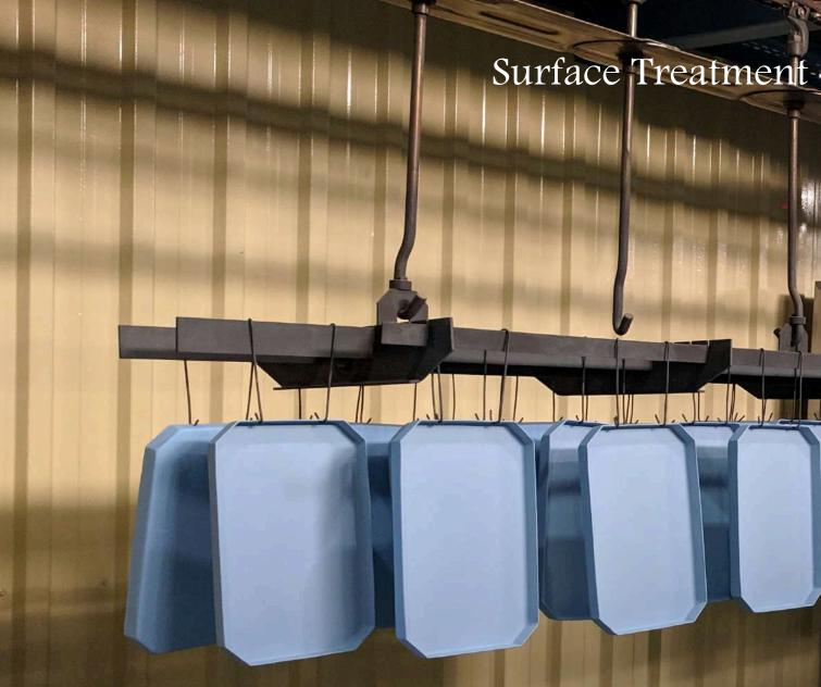
We provide multiple methods of surface treatment options for architectural and decorative metal structures, those methods include Hot Dip Galvanizing, Thermosetting & Thermoplastic Powder Coating, Vitreous Enameling, Electroplating and Wet Paint.
